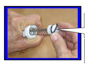
Installing O-rings onto plunger F **0491**
