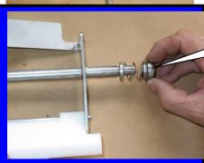
Step 5: Install spring seal **F0355**
