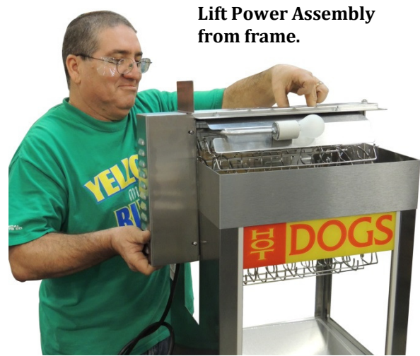
Removing/Reassembly of Power Assembly
