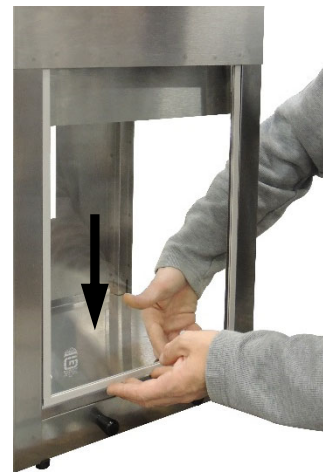
Lower glass panel into bottom channel.
